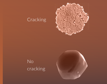
Exhibit B Commercialized polycrystalline cathode particle (top) and single crystalline cathode particle (bottom)
